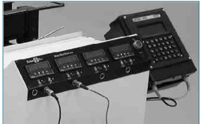
Close up of High Load Interface Shear Box,
